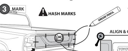
**DRAW CENTER HASH MARK WITH GREASE PENCIL ON APPLIQUE AND** SHEET METAL, THIS WILL ENSURE **APPLIQUE WILL BE CENTERED TO GREASE PENCIL OUTLINE.**
